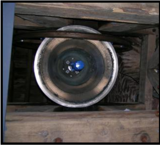
One of the bells showing where the bronze has been removed in order to tune it to the correct note.
